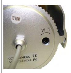
When making Zoom and Focus adjustments, STOP when there is a slight resistance. Forcing the camera's adjustment will void the warranty and damage the camera
